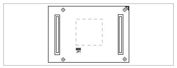
Figure 12 JP1 Jumper Socket
